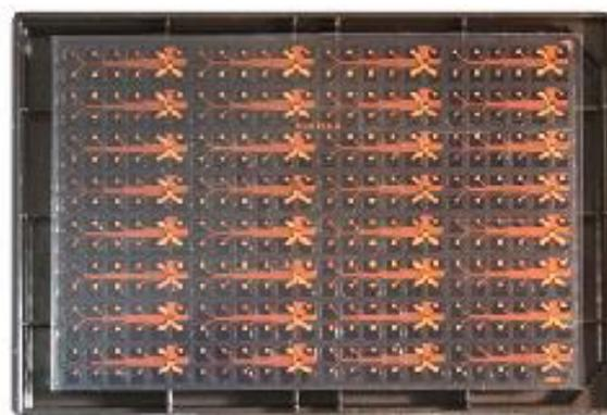
The IonFlux plates are based on the 96 or 384 SBS-standard format. (Left) an IonFlux HT system capable of 64 parallel recording. (Right) the microfluidic network attached to the bottom of a 384 well plate. This plate is used with the IonFlux HT
